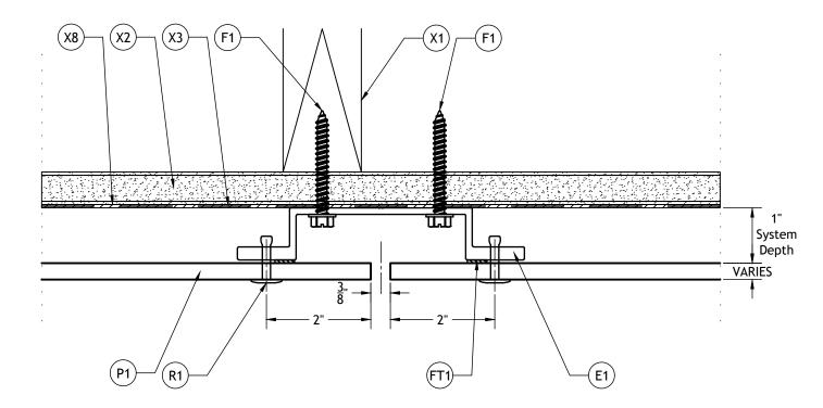
Note: The extrusion fasteners (F1) for each hat channel extrusion (E1) alternate positions along the length of the extrusion. The two alternating positions are shown in the drawing above.
